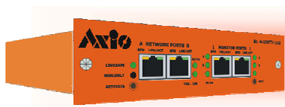
The AxioTAP Class A3 - Gig LinkSafe TAPs are ideal for undetected, fail-safe monitoring of full duplex Fast and Gigabit Ethernet Network data transmission traffic. High Availability model is also available for deployments in redundant network configurations.
